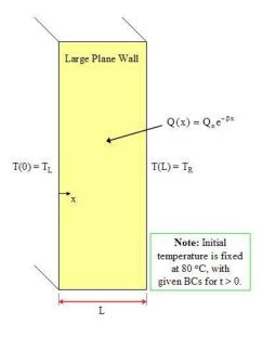
Now, your task for this problem is to evaluate the above expressions for T(x,t) and to plot the resultant space-time temperature distribution, as appropriate, so that one can easily visualize the time-dependent temperature distribution within the wall, both quantitatively (with a 2-D plot containing  $T(x,t_i)$  for several time points,  $t_i$ ) and qualitatively (with one or more 3-D views) -- and be sure to properly label your plots. Rationalize that your solutions physically make sense!
