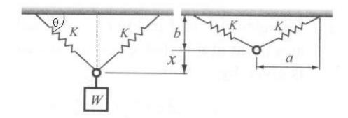
The weight of the object placed on the scale can be expressed in terms of the vertical distance, x, by performing a force balance on the system with the weight, W, included. For equilibrium, the downward force due to the weight must be balanced by the upward force due to the springs, or
