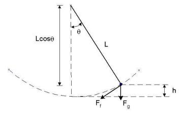
For a pendulum of fixed length, the radial acceleration is zero; thus there is no motion
