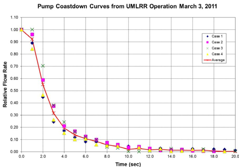
**Fig. 4 Pump coast-down curve for the UMLRR primary pump.**
