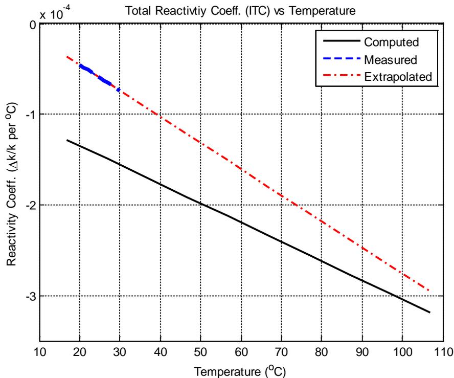
**Fig. 3** Calculated and measured isothermal temperature coefficients for the M-2-5 core.
