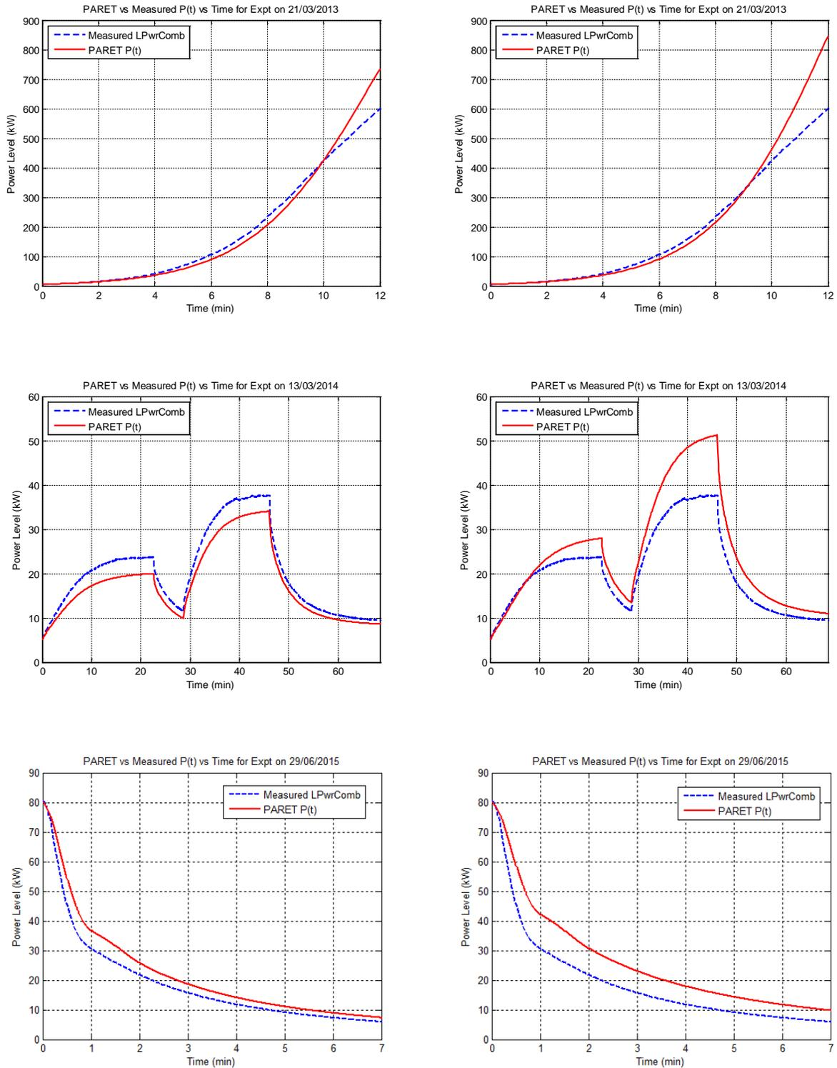
**Fig. 10 Selected results with nominal (on left) and reduced (on right) reactivity coefficients.**
