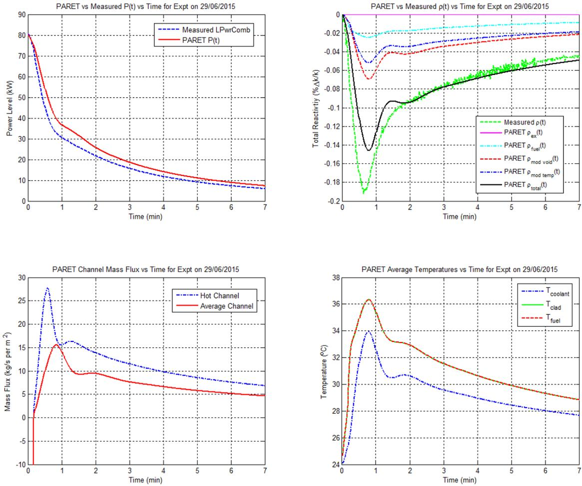
**Fig. 8 Summary results for the pump-off test from June 29, 2015 with  $P_0 = 80$  kW.**
