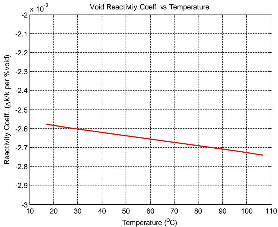
**Fig. 2** Calculated void reactivity coefficient vs. temperature for the M-2-5 BOL core.
