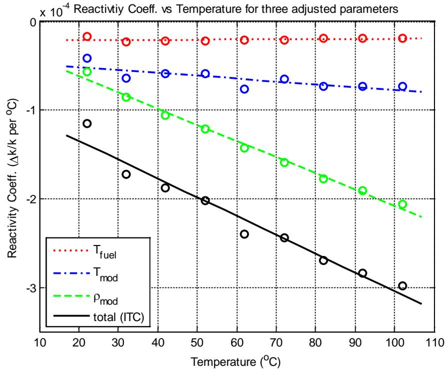
**Fig. 1** Calculated reactivity coefficients vs. temperature for the M-2-5 BOL core.
