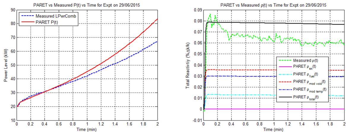
**Fig. 9 Summary results for the pump-on test from June 29, 2015 with  $P_0 = 20$  kW.**
