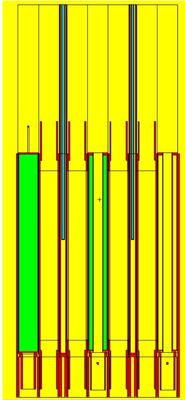
Fig. 12 Full YZ view of UMLRR M-1-3 core model ( x = 10 cm).
