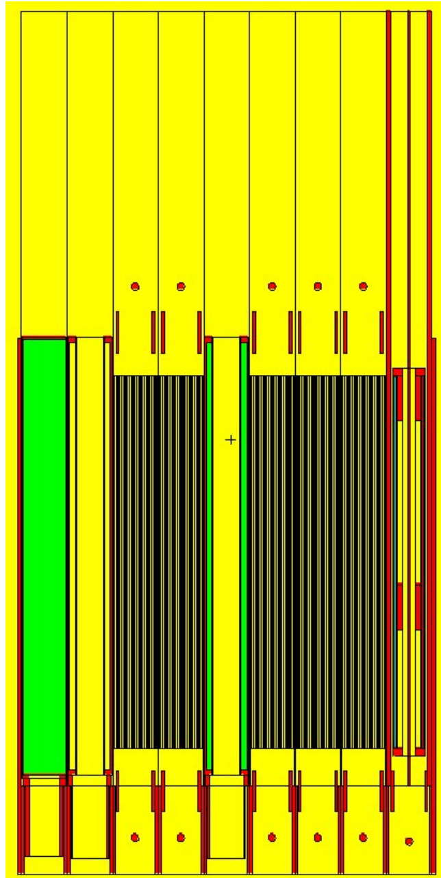
Fig. 11 Full XZ view of UMLRR M-1-3 core model ( y = 23 cm).
