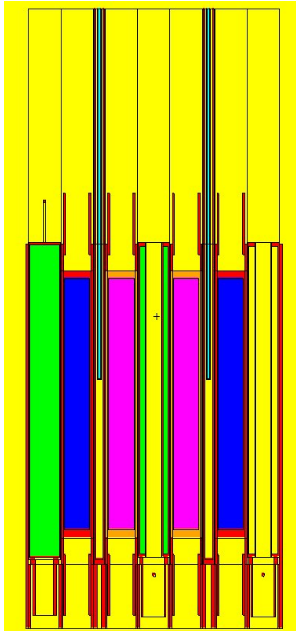
Fig. 13 Full YZ view of UMLRR M-1-3 core model (x = 10.17 cm).
