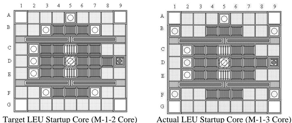
Fig 2. Target and actual LEU startup core designs for the UMLRR.
