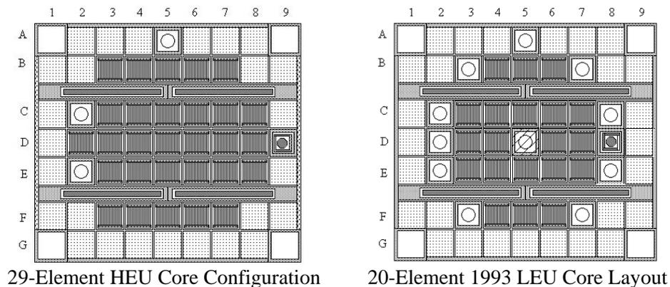
Fig 1. HEU reference and preliminary LEU core designs for the UMLRR.
