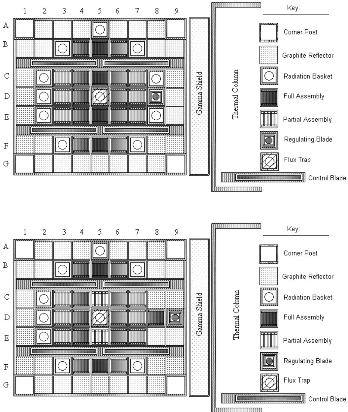
Fig. 1 Original (top) and new (bottom) reference LEU core configurations.
