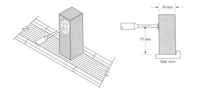
One part of an inspection system in a packaging operation uses a jet of air to remove imperfect cartons from a conveyor line.
