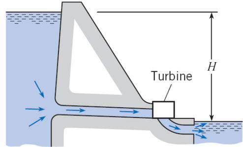
2. Water flows through the horizontal pipe shown below at a rate of  $7.85 \text{ m}^3/\text{s}$ . The pipe inside diameter is 1 m. The head loss coefficient in the pipe was measured to be about 7.0 based on the velocity head in the pipe.
