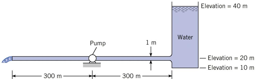
3. Consider the situation identified in the diagram where water is drawn into the pump as shown. The pipe inside diameter is 4 inches on the suction side of the pump and 3 inches on the discharge side and the remaining data for the problem are given below:
